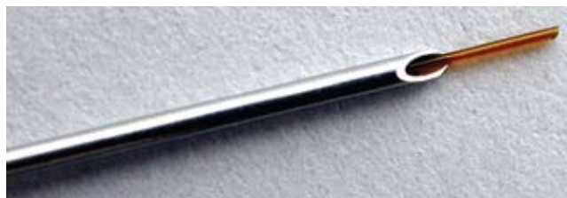
Fig. 4. Photograph of a 20-gauge spinal needle with the fused silica catheter prior to stereotactic insertion. The spinal needle serves as a linear guide and a protective sheath for rigid fixation.
